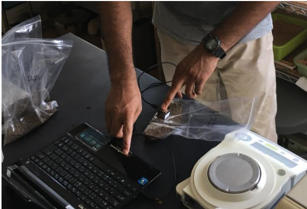
Photo 3: Measuring the reflectance spectra (between 1550 and 1950 nm) from soil in the laboratory with an inexpensive handy-held Spectral Engines NIRONE Sensor S2.0.
