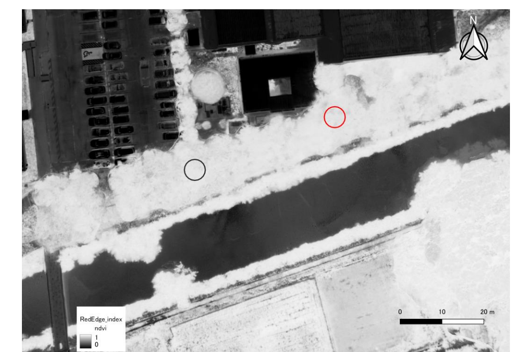
Fig.3. NDVI image calculated from RedEdge-MX
