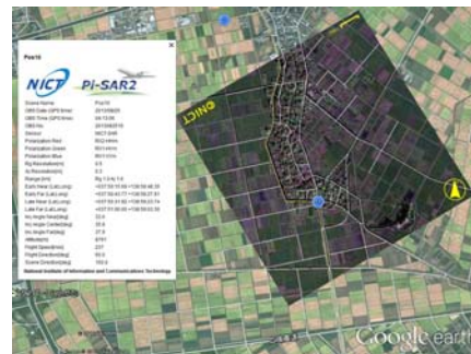
Fig. 4. Onboard processed and transferred KMZ observed on 25 Aug., 2013. The size of image is 1 km × 1 km. Observational and geographic information is shown in the balloon.
